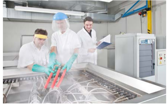
Fig. 06-20 In the endurance test, the pipes are tested for their temperature and pressure resistance
