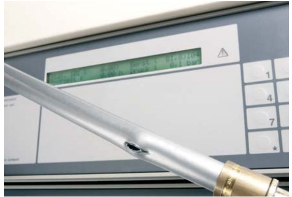
Fig. 03-8 Burst pressure test
