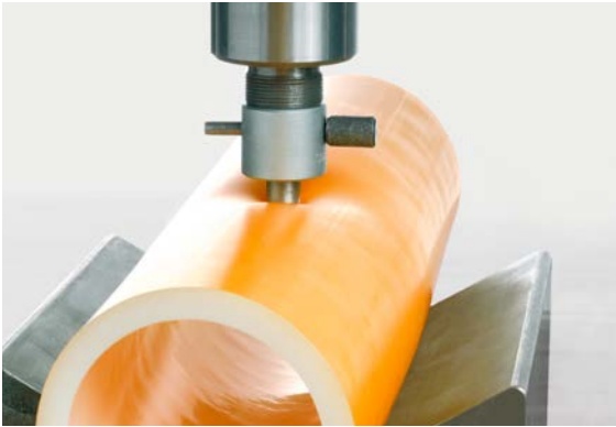
Fig. 03-6 Point load test
