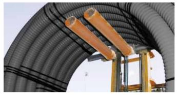
Fig. 41 Lifting with a forklift
