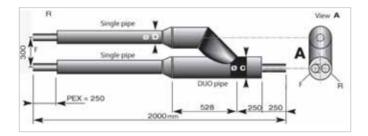
Fig. 53b Transition from UNO to DUO pipe using prefabricated Y-pipe
