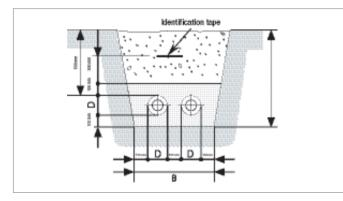
Fig. 33 Pipe system with UNO pipe
