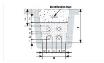
Fig. 34 Pipe system with UNO pipes laid above one another
