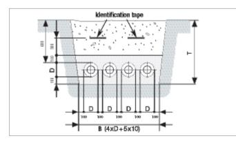
Fig. 35 Pipe system with UNO pipes laid next to one another
