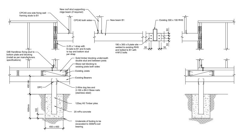
ROOF BEAM B1 DETAIL
