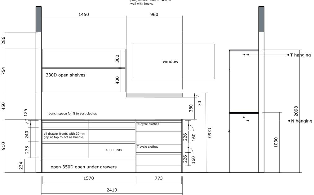
5 dble coat hooks for caps @ 200ctrs pine/melteca board fixed to wall with hooks
