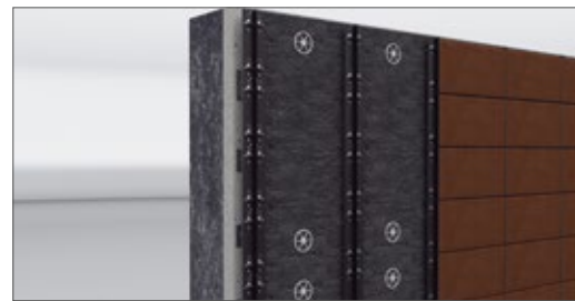
Mount the T-profile with approved fastening means
