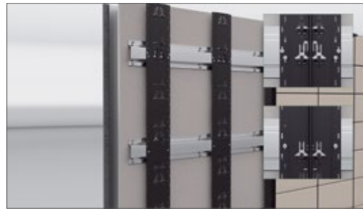
Fasten Omega profile with Al blind rivet (Art. no. 658) or A4 stainless steel screw (Art. no. 659) (Pay attention to fixed and sliding point)
