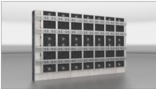
Basic substructure with K20 Omega profiles
