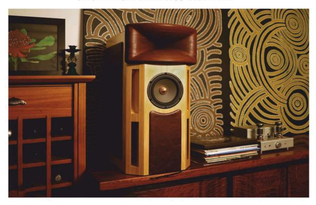
that driver visible on the front baffle as a 'mid-bass'. Well, it's simply that it is neither a midrange driver nor a bass driver, but a bit of both.
