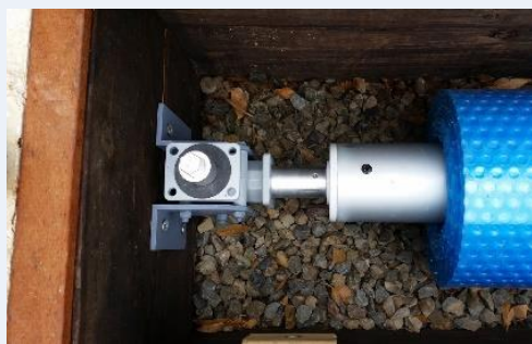
Roller tube mounted to gearbox
