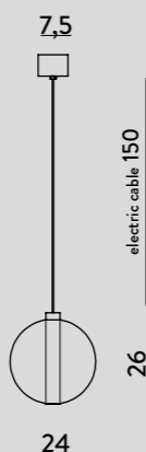
GIG1293.1L SOSPENSIONE / HANGING LAMP Glass Ø24 cm - cavo/cable 150 cm G9 1 x max 42W 230V CE IP20 1m
