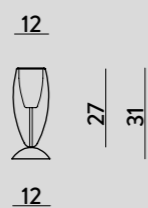
LU1390.1L LAMPADA DA TAVOLO / TABLE LAMP Glass Ø12 cm - H 31 cm E14 1 x max 60W 220-240V CE IP20 1m
