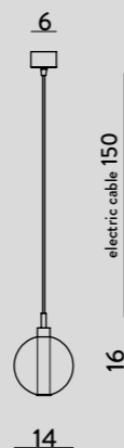
1293.1L SOSPENSIONE / HANGING LAMP Glass Ø14 cm - cavo/cable 150 cm G9 1 x max 42W 230V CE IP20 1m
