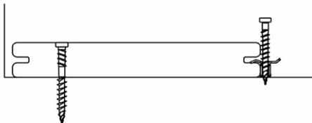
STEP 2: Use a hidden fastener in the groove of the board.
