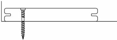
STEP 1: Fasten your first deck board with a starter clip, or composite deck screw. Pre-drilling of screws gives best results, and is required within 50mm of the end of a board.
