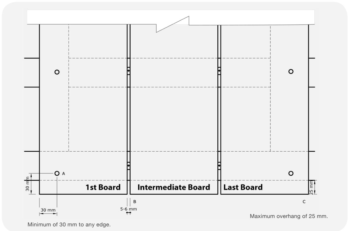
Note: All fasteners within 50mm on the end of the board requires pre-drilling.
