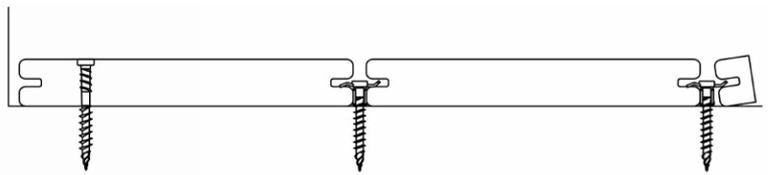
STEP 4: Insert the next line of hidden fasteners and follow with the next board.
