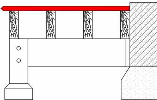
Should the board be pressed against the edge of a wall, then the board will move in the opposite direction.
