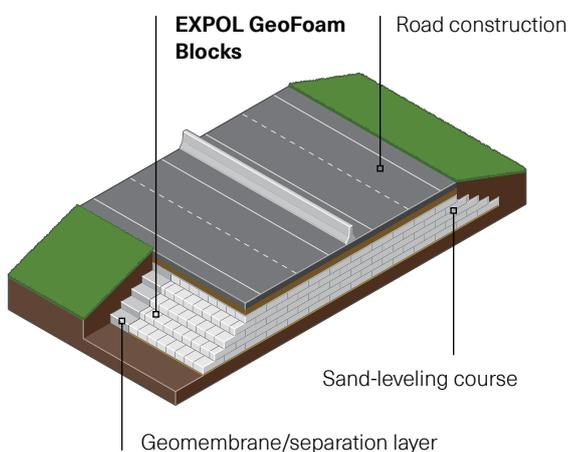
The roading system, which generally consists of select fill, road base gravel and an asphalt or concrete driving surface, is subsequently constructed atop the separation layer. Prevention of differential icing is a consideration when using EXPOL GeoFoam in roadway construction in cold climates.
