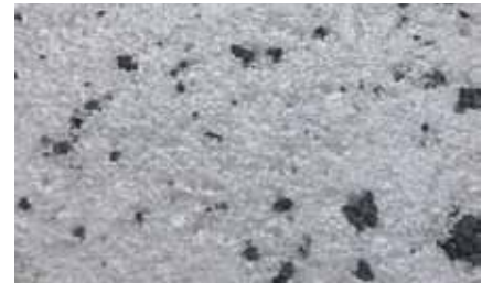
EXPOL StyroDrain is made from 100% Recycled Polystyrene
