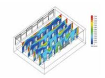
**Figure 6** Air velocity distribution around the occupants
