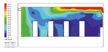
**Figure 5** Air velocity distribution for high level tophung outward opening windows
