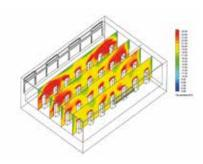
Figure 3 Temperature distribution around the occupants
