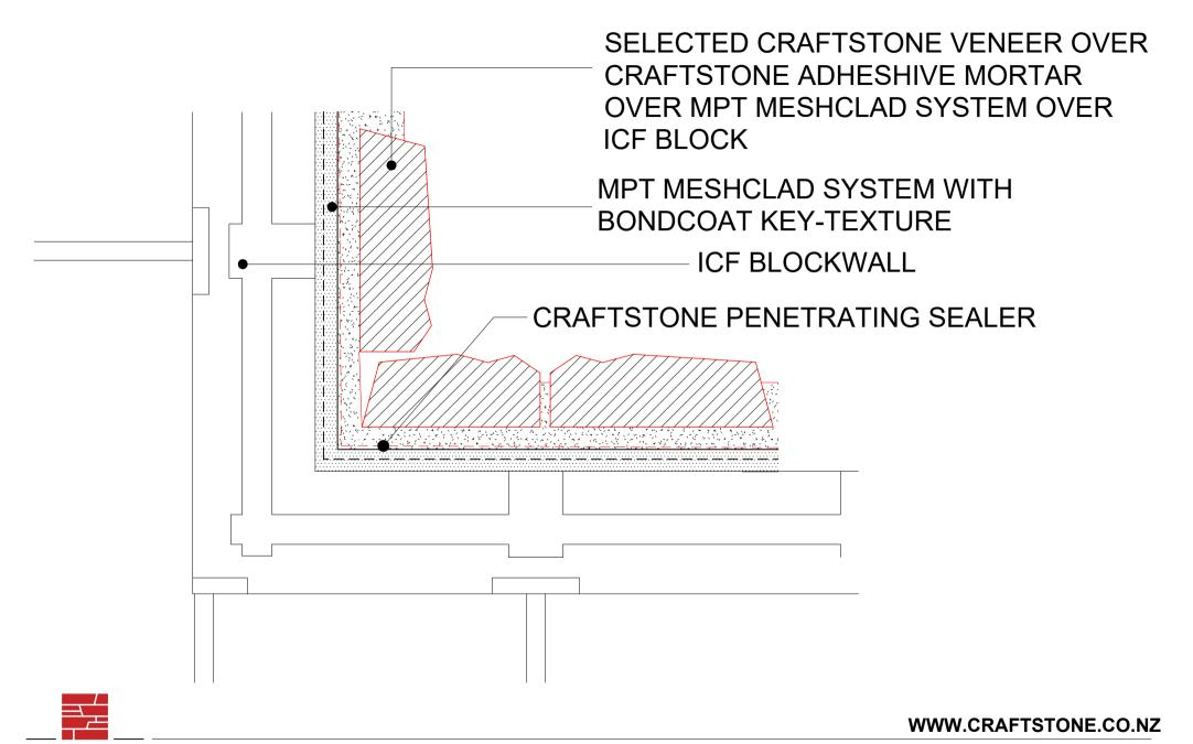
CR AFT TYPICAL INTERNAL CORNER DETAIL
