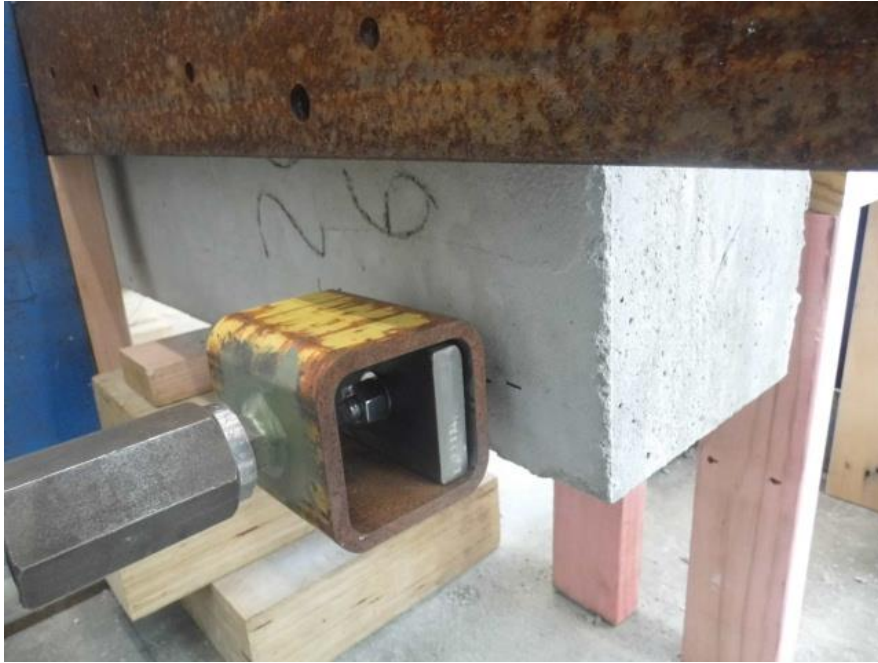
Photograph 7. Steel fitting used for axial tension tests (without bottom plate)
