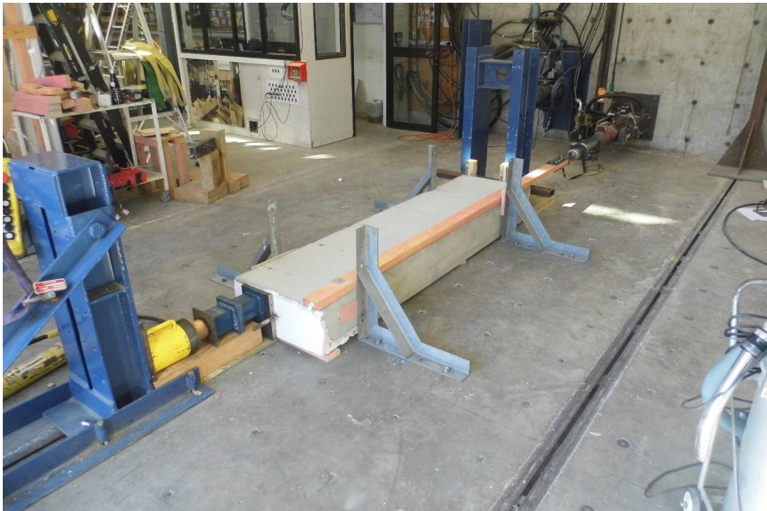
Photograph 4. Set-up for in-plane tests
