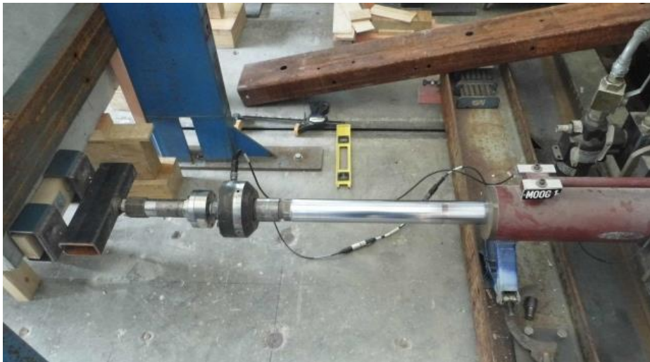
Photograph 6. Test set-up for axial tension loading (bottom plate anchors)
