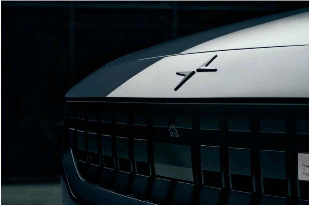
Polestar emblem is colour coded to match each Polestar 2 body colour. The Grid is Polestar's answer to the traditional front grille. This is where Polestar integrates its sensor technology including the 360° camera (Pilot lite pack) and the radar sensor.
