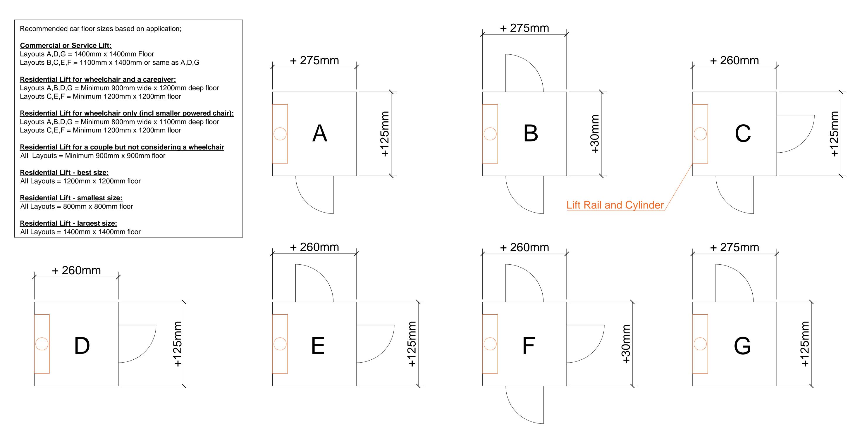
To use this Lift Shaft Size Guide to calculate your LIFT SHAFT size, add the numbers on each layout to your desired floor size
