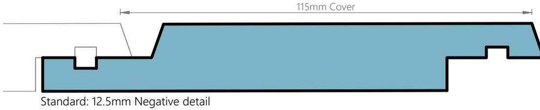
P52 Bevel Grooved Vertical Shiplap Profile
