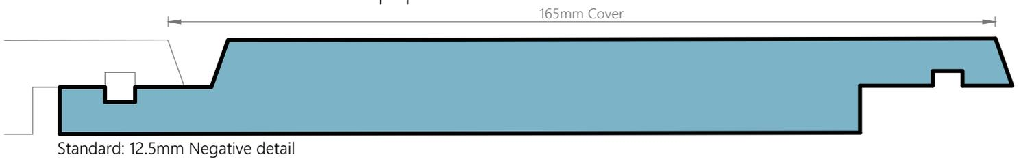
P53 Bevel Grooved Vertical Shiplap Profile
