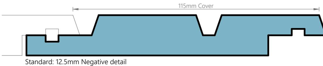
P54 Bevel Grooved Vertical Shiplap Profile
