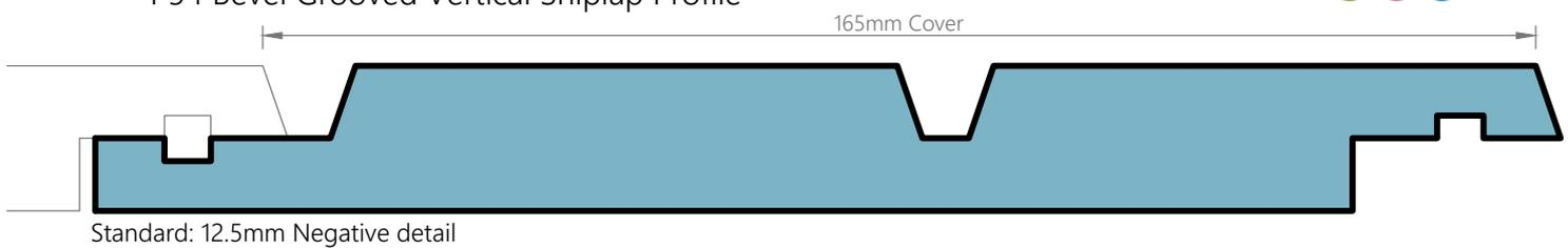
P57 Bevel Grooved Vertical Shiplap Profile
