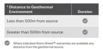
\* Distance from bore, mud pool, steam vent, or other source with a pH between 5 and 9. For a pH outside this consult Dulux.
