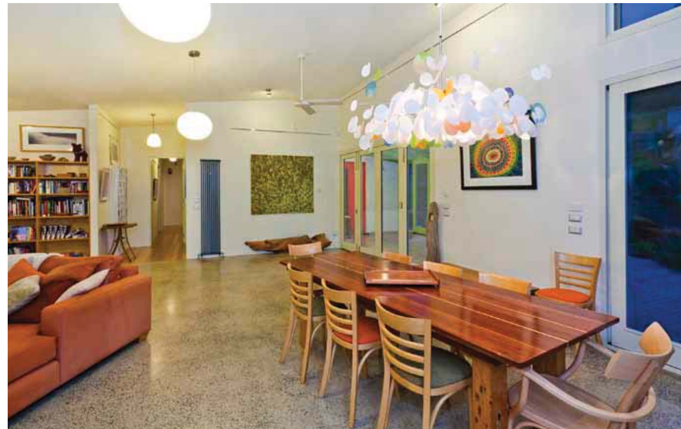
Cooling and heating of the living and dining rooms is aided by the attached wintergarten to the north. The double glazed doors of the wintergarten are visible in the centre of the image.
