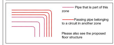
Only connecting lengths to and from floor loops are are allowed to cross construction joints. Pipes which do cross joints must be
