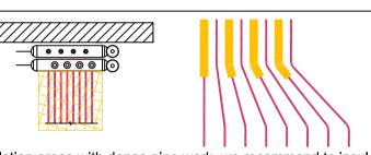
In installation areas with dense pipe work, we recommend to insulate part of the pipe work with corrugated conduit until the pipes reach the design pipe spacing.
