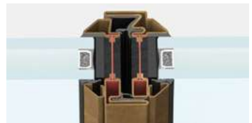
central section | frame section 62 mm
