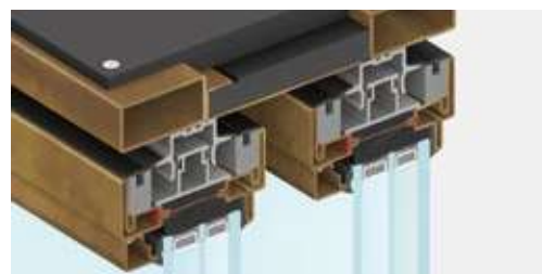
floor rail with threshold | h 8 mm
