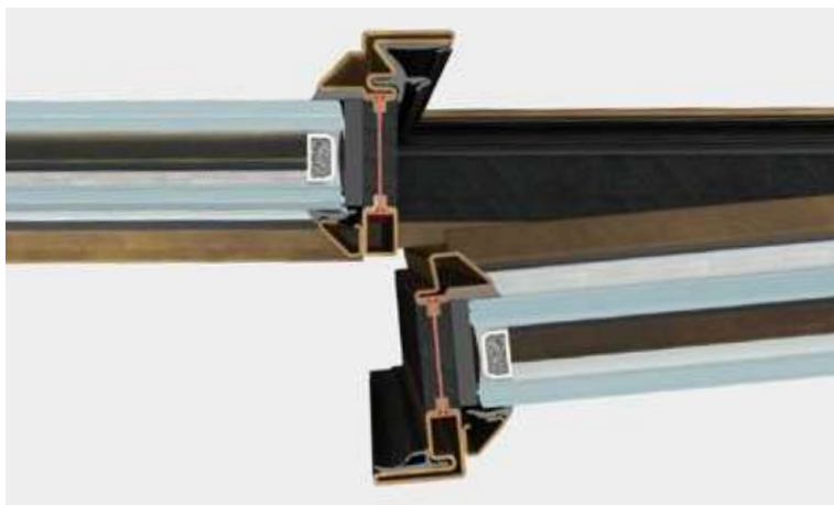
central section | frame section 62 mm
