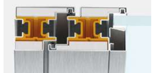
lateral section | frame section 134mm
