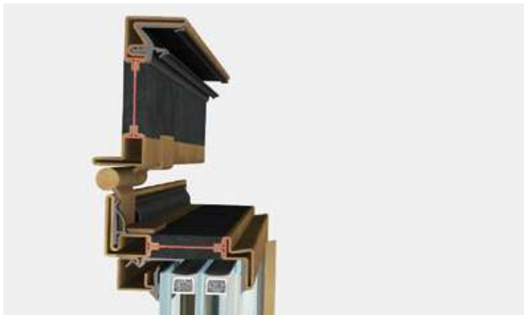
lateral section | frame section 47 mm
