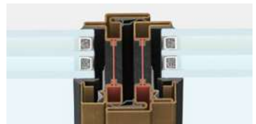
central section | frame section 62 mm
