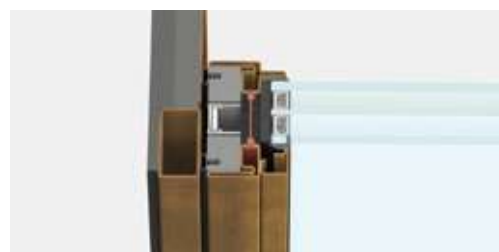
standard central section | frame section 94mm
