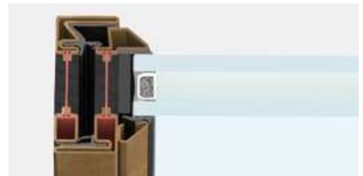
lateral section | frame section 47 mm
