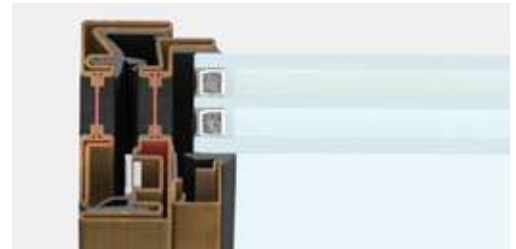
lateral section | frame section 47 mm
