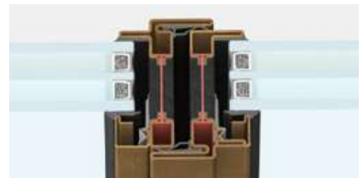
central section | frame section 62 mm
