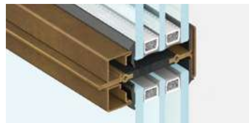
glazing bar | frame section 36 mm
