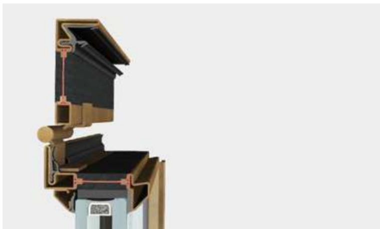
lateral section | frame section 47 mm
