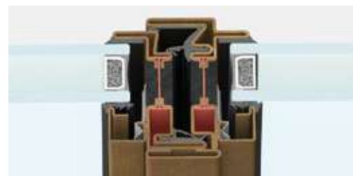
central section | frame section 62 mm
