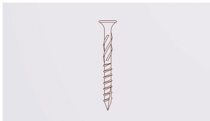
Abodo Stainless Steel Cladding Screw 4.0 x 45mm or 4.5 x 65mm:
