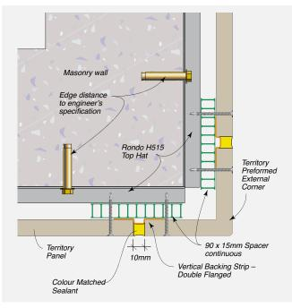
FIGURE 8.43 External Corner Detail – With Coloured External Corner Trim – Plan View
