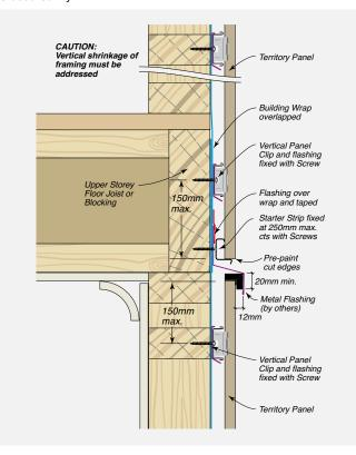
**FIGURE 8.19** Horizontal Control Joint – Between Panels
