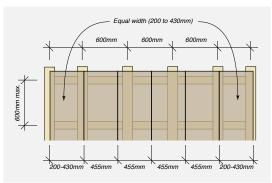
FIGURE 7.03 Symetrical Panel Set-out – Steel Framing
