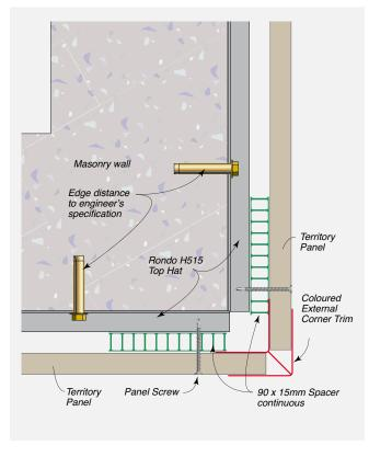
FIGURE 8.44 Internal Corner Detail – With Backing Strip and Colour Matched Sealant – Plan View
