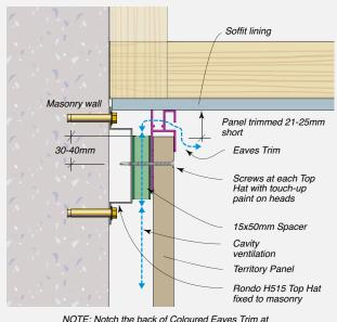
NOTE: Notch the back of Coloured Eaves Trim at intersections with Joint Backing Strip
