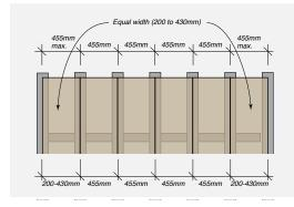
Note: For framing other than 455mm centres, horizontal structure members can be used (eg. top hats and additional timber framing). Contact DesignLink for further information.
