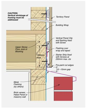
FIGURE 8.03 Base Detail - Beam & Joist Construction
