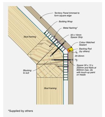
Note: Drawings are interchangeable for timber or steel substrates with the exception of the fasteners.
