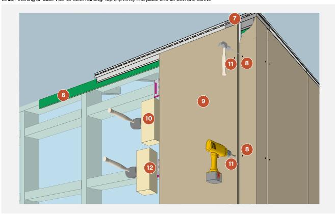
(a) Lift the next panel into position, placing the head into the soffit trim and base onto the starter strip. (a) Slide the panel into the existing clips. Firmly tap panel into position. (b) Fit and fix panel clips and panel clip flashings to the framing as for the previous clips. Repeat steps (b), (c) and (b) for additional panels. (c) Mask and prime edges of expressed joint and fill joints with colour matched sealant. Prime and touch-up visible fixing heads.
