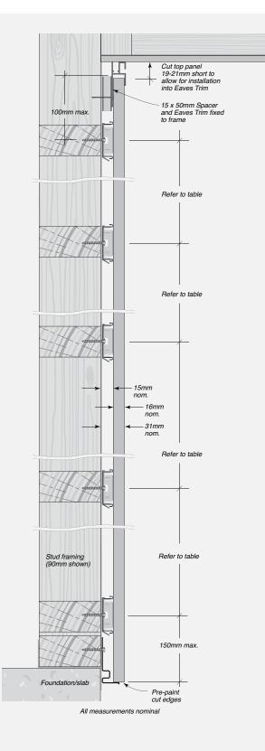
FIGURE 7.06 Typical Territory System Cross Section - Elevation
