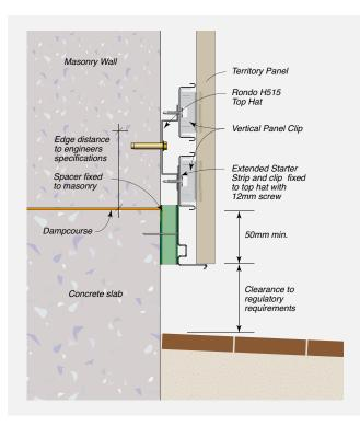
FIGURE 8.39 Base Detail - Concrete Slab Construction - Plan View
