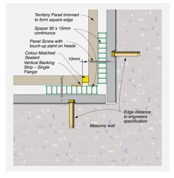
FIGURE 8.45 Parapet Detail - Elevation
