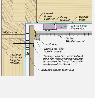
FIGURE 8.35 Typical External Corner Junction Panel to Weatherboard - Plan View
