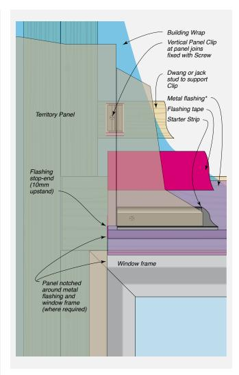
Note: Drawings are interchangeable for timber or steel substrates with the exception of the fasteners.
