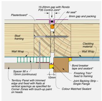
FIGURE 8.37 Typical Abutment with In-set Masonry Wall - Plan View
