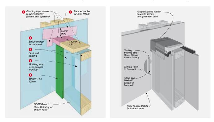
FIGURE 8.26 Two Sided Parapet Wall Junction – Stage 1 Procedure
