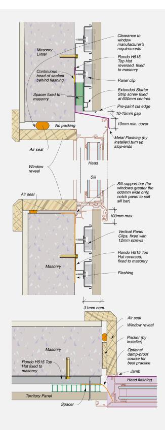
Note: Drawings are interchangeable for timber or steel substrates with the exception of the fasteners.
