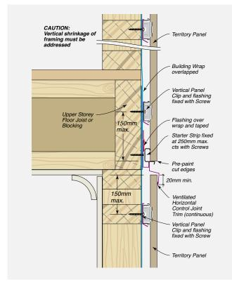
FIGURE 8.20 Horizontal Control Joint – Second Storey Junction – Closed Cavity
