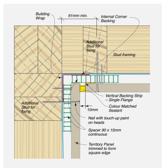
FIGURE 8.09 External Corner Detail – With Coloured External Corner Trim – Plan View
