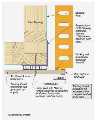
FIGURE 8.31 Internal Corner Junction – Panel to Brick Veneer Plan View
