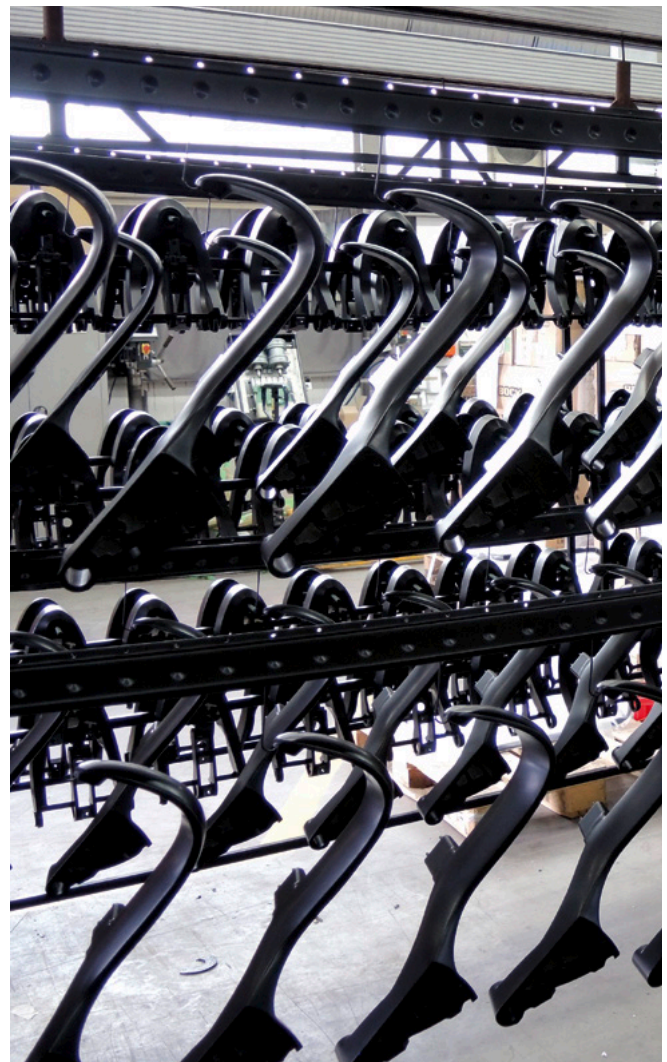
Before powder varnishing, each part is checked to ensure the surface is perfect and other quality characteristics have been complied with.
