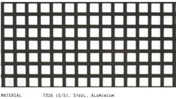
MATERIAL T316 (S/S), STEEL, ALUMINIUM MAX WIDTH 1200 OPEN AREA 53% THICKNESS 1.0-2.0MM (S), 0.9 -1.5 (S/S), 1.0-3.0MM (A) STOCK STATUS CUSTOM MADE
